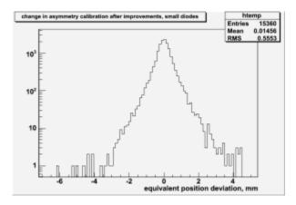
For some crystals the improvements was significant, while in average the effect is modest (about 0.5 mm).
