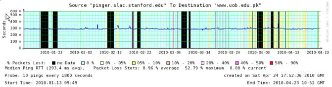
It is seen that though it's reachability is not great it is responding most of the time. I am able to get partial data from it for the last few days using getdata\_all. pl. This is reflected in its collection status.
