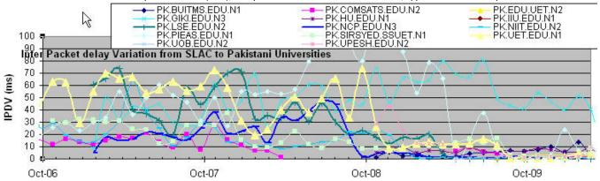
The improvement in the PingER IPDV between SLAC and NCP (moved to TEIN3) and SLAC and PERN (not moved to TEIN3) can be seen in the plot below. It is seen that both have improved with time, though the improvement for NCP is much more dramatic. Both are now small and comparable and < 2
