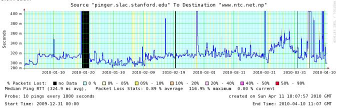
So we could compare the above measurements with those of a host connected to TEIN3 we added www.nren.net.np as a "Beacon" to the list of PingER monitored hosts on 4/17/2010. The traceroute from SLAC to it identified it as being connected to TEIN3.
