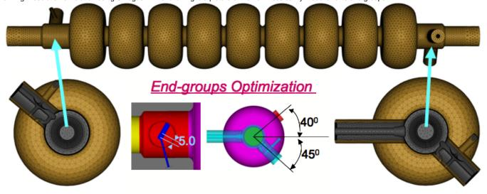
We optimized the end-groups using Omega3P and provided an improved design. The following is the comparison of Q and R/Q for the original design and the improved SLAC design.
