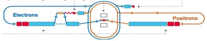
Each Main Linac will have a dual-tunnel configuration, one for acceleration and the other for service. In the acceleration tunnel, there will be about 20,000 superconducting cavities chained together to provide the acceleration of electrons or positrons to 500 GeV. The following is a schematic picture of the dual-tunnel configuration.
