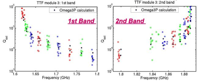
The above picture shows that the measured external Q's are scattered round the computed ones. This is due to the deformation of the cavities. We have developed a method to compute the deformation from the measurement data, through an inverse problem approach.
