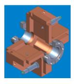
Heating Study for SNS Cavity with HOM Couplers (Under Construction)
