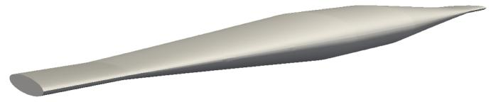
Wakefields of Undulator Taper with a 0.5mm bunch is calculated with 6000 cores and 12 hours. It used 0.25 mm mesh element size with 19 million quadratic tetrahedral elements for the whole geometry. The left hand side is the wakefield due to a 0.5 mm bunch while the right hand side is the comparison between the reconstructed wakefields of a 3 mm bunch from the wakefields of 0.5 mm bunch and the calculated wakefields for a 3 mm bunch. The comparison shows that they are in a remarkable agreement.
