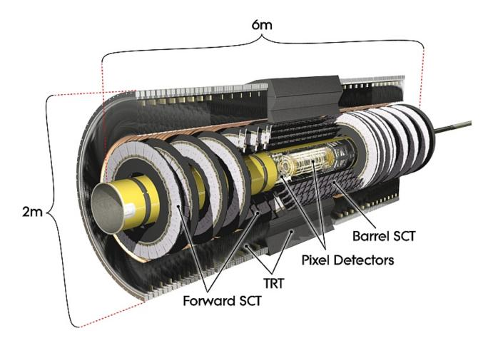
The inner detector is composer of three separate sub-systems: Pixel, SCT and TRT.
