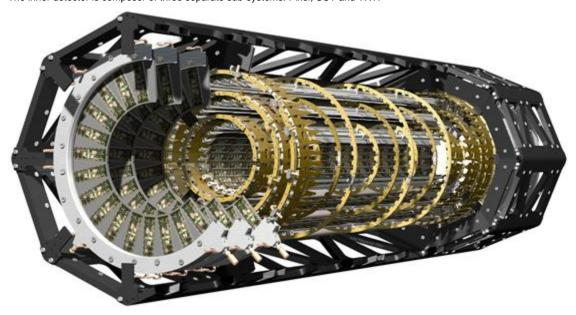
This image shows a cross-section view of the pixel detector only. One can see the three barrel layers, and the three disks
