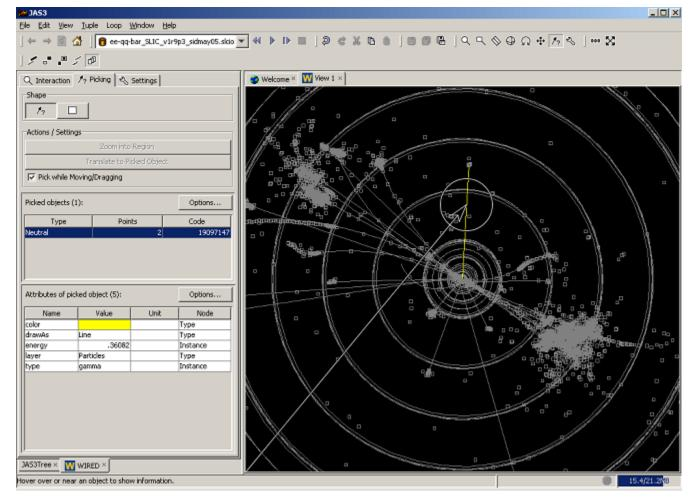
The tracks HepRep attributes are displayed in the window. For instance, my selection is a gamma particle with energy of 0.36082 GeV.
