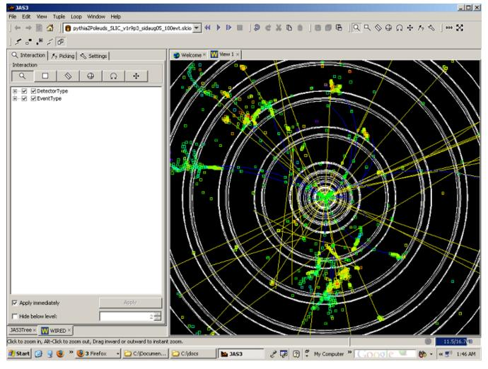
The detector geometry is drawn in white on the black background. (In general, structures within the detector such as layers and sublayers are left out to improve performance and reduce visual clutter.)
