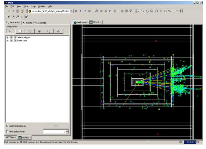
The XY projection is a front or beam view, which is the same as the view when the LCIO file was first loaded.
