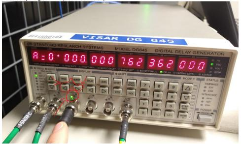
3. With the "A" channel selected, use the "CURSOR" left and right arrows (circled below) to ensure the flashing digit corresponds to the decimal place desired for adjustment. (Oftentimes adjustments on the order of single nanoseconds is needed, so the flashing digit should be the one circled below.)
