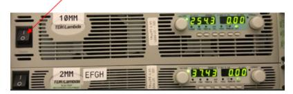
1. Press the tiny "out" button at each of the 4 supplies. The green LED above the button should then be illuminated
