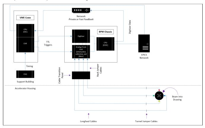
(Figure 1- Setup for VME based BPMs, note that the VME crate sends forward communication to the BPM chassis through the use of TTL triggers. The AFE (Analog Front End) of BPM chassis receives raw beam
