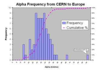
The median value of alpha from CERN to Europe is 32.55 (km/ms). The IQR is 11.61 km/ms or IQR/Median~ 36% or ~ +-18%. The maximum value for alpha is 87.55 Km/ms (CERN to EPFL) which is because CERN and EPFL are only about 100 km away from each other, so selecting the highest value of alpha in this case may be mis-leading.
