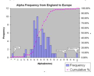
The median value of alpha from England(Warrington) to Europe is 40.71 (km/ms). The IQR is 15.6 (km/ms) or IQR/Median~ 38% or ~ +-19%. The highest value of alpha 97.72 (km/ms) is due to a very small RTT (2.6ms) between (demon.co.uk) and this landmark which are 263 km apart.
