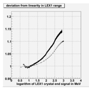
One can see that at high signals (300-1000 MeV) the deviation from linearity measured by real events is ~5% bigger than one measured by charge injection.
