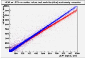
One can see that non-linearity correction is up to 10 % and definitely inproves the situation. Without correction LEX1 energy would be ~10% bigger than HEX8 energy at the end of the range.
