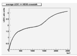
The effect of this crosstalk is substancial for very low signals. To account for it I subtracted this crosstalk from on-orbit data (as the plot give xtalk in HEX8 adc vs LEX1 adc I can do it directly.
