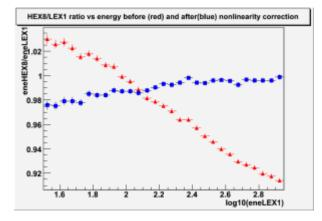
Red points shows the HEX8/LEX1 ratio without nonlinearity correction, blue points - after standard nonlinearity correction with charge injection spline used actualy in reconstruction.
