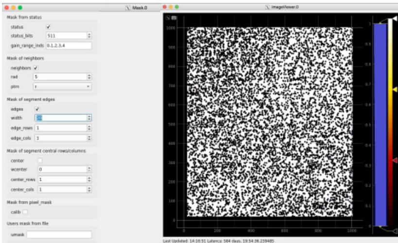
Adjust the mask parameters using editor window and click on "Apply" button again. Mask image will have changed according to set parameters.
