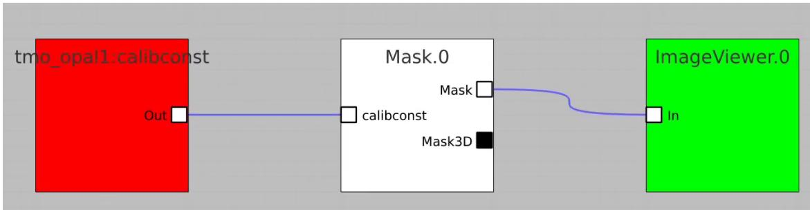
Click on "Apply" button, then click on Mask.0 and ImageViewer.0 control nodes to open editor for mask parameters and mask image viewer.
