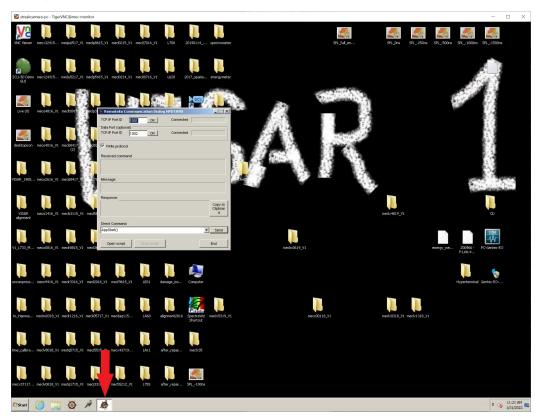
• Pull up the "Long pulse laser operation" screen, and make sure the "StrkCam" is enabled ("DIS" shows as the button option) and the trigger rate is non-zero. If it is zero, hit the "5 Hz" button to start generating triggers. (Remember to reset the mode after the IOC has been correctly started.)
