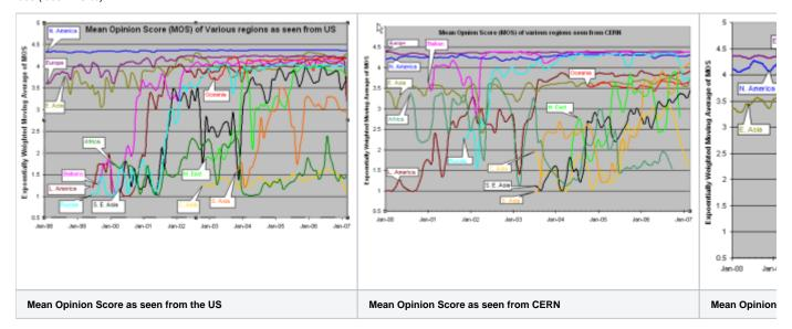
CERN monitors fewer remote hosts than SLAC (56 versus over 400) so the data is not as complete in the CERN case. Comparing the two graphs, it can be seen that, as expected, the MOS is better for the shorter distances (i.e. CERN to Europe is better than SLAC to Europe, SLAC to N. America is better than CERN to N. America.).
