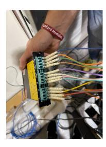
We decided to avoid connections on the DPM6 as this particular RCE showed few errors during testing. To do so we used a breakout box to re-map the data connections.
