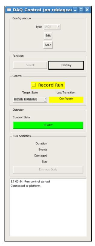
You can stop the run from the control gui window by selecting one of the available Target States from the box in the Control Panel. The states are "disable", "end running" or "shut down".
