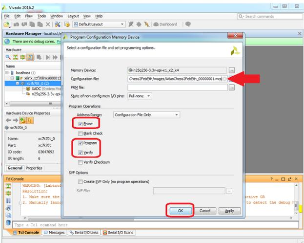
6) After your done loading the PROM, you can either power cycle the carrier board to load the new image from the boot PROM to the FPGA or "Boot from Configuration Memory Device" via the JTAG interface
