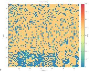
09:30 FE65-P2: ran tune\_globalthreshold and tune\_pixel threshold and got okay results from an analog scan:
