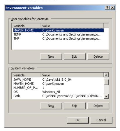
After installation, also set the MAVEN\_HOME variable to point to the base installation area.
