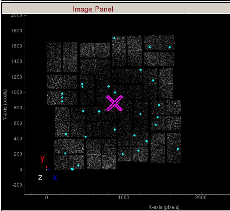
Indexed peaks are shown in magenta. Peaks found are shown in cyan. Each indexed peak are represented by the integration rings. The unit cell parameters are displayed on the side. A failed indexing result will be displayed as a big X.
