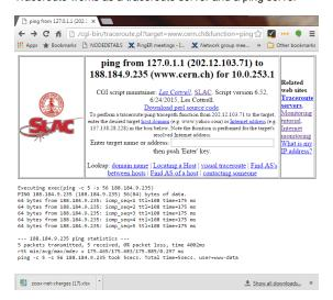
Looking at the function=ping output, you will notice that the requesting host (in this case at SLAC) is given a private IP address (10.0.253.1) which is going to cause some failures, e.g. a host at SLAC requesting a ping from 202.12.103.71 to the requesting host. The requesting host being identified as a private address 10.0.253.1 will not be able to be pinged. See below:
