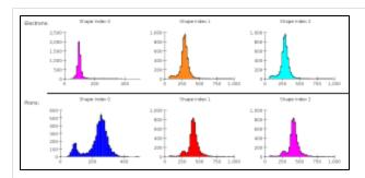
The first three values of the getShape() parameter for electrons and pions using only the highest energy cluster with no timing or energy cuts.
