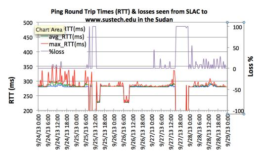
The loss of connectivity (RTT=unknown=0, loss=100%) is seen between 8:00 and 8:30am September 25th GMT, there is a recovery between 9:00 and 10: 15, and then a further loss of connectivity until 13:00. The drops in minimum RTT from ~280ms to ~230ms is probably due to the use of an alternate route. Below is another plot of the data.
