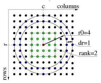
When peak is found, its parameters can be precised for background level, noise rms, and signal over background ratio (S/N) can be estimated. All these values can be evaluated using pixels surrounding the peak on some distance. For all peak-finders we use the same algorithm. Surrounding pixels are defined by the ring with internal radial parameter r0 and dr (both in pixels). The number of surrounding pixels depends on r0 and dr parameters as shown in matrices below. We use notation
