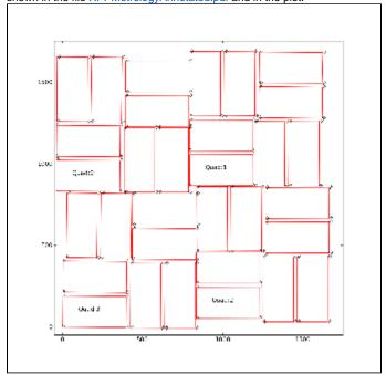
The 1-st corner of the 3-rd quad (x,y,z) coordinates are re-set to (0,0,0) in the beginning of measurements. At the end, it is checked that the 1-st point coordinates are reproduced within precision of measurement.
