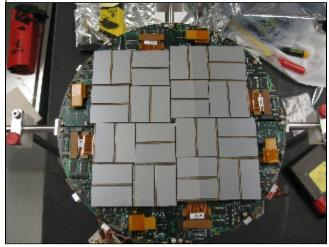
Pixel coordinates in 2x1 sensor chip are known with sub-micrometer precision. Construction of the detector allows significant freedom in relative positions of 2x1 sensors. To get precise pixel positions in the detector the 2x1 sensor coordinates needs to be calibrated. In this note we describe geometry of the CSPAD detector, optical and quad alignment procedure, parameters, and software providing access to precise geometry information.
