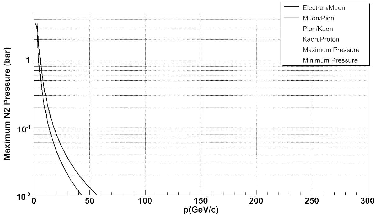
6 meter long Cherenkov efficiency as a function of the beam momentum to select different particles
