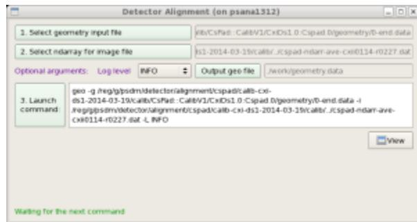
Alignment tool works with `geometry` files, produced in Metrology tool and allows to tune quad or other sensor positions in the detector, using image with real objects (rings, shadows, etc).
