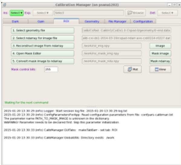
The files with ndarray and geometry constants should be selected as input parameters in the first two options of this GUI. The names of other intermediate and output files for "Image", "Mask image", and "Mask ndarray" are optional. Next three buttons
