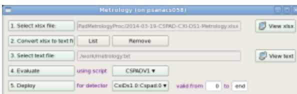
Metrology tool processes `xlsx` files from optical measurements, produces calibration constants of types `geometry`, `center` and `tilt`, and deploy them in calibration directory.
