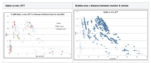
The red dots are the points for monitor AIOU, the green dots are for the remote UAF. The downward sloping lines are for monitor-remote hosts separated by roughly the same distance, e.g. monitors and remotes in Karachi and Lahore.
