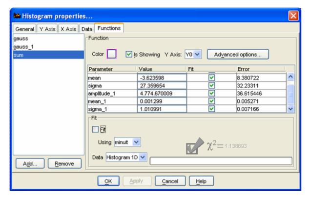
Through this dialog it is possible to choose which optimizer engine is used in the fit, control the parameters value and also fixing them by unchecking the appropriate checkbox under the *Fit* column next to the parameter's name.
