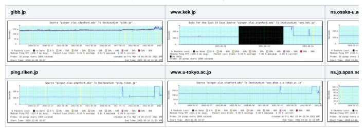
Looking again on April 5th 2011, the RTTs from SLAC to the University of Osaka, RIKEN, University of Tokyo and KEK all increased with a step function from around 135ms to around 200ms around midday on the 24th March. Below is shown the RTTs for RIKEN as an example.
