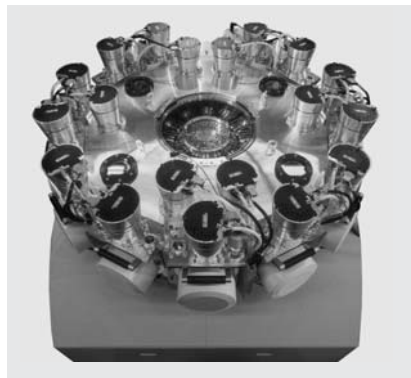
Entire high vacuum equipment of a CD/DVD coating system with TURBOVAC TW 250 S pumps
