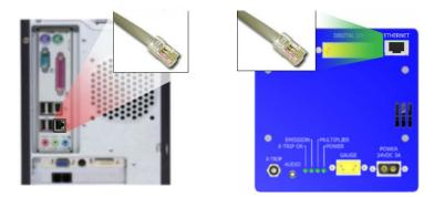
Connect the 24VDC 2-pin D-type to the socket labeled "Power", connect the IEC mains lead to the 24VDC power supply and finally connect to your local mains supply.
