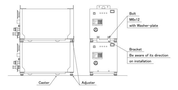
Fig. 4.4 Piling two pumps
