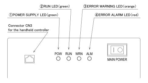
Fig. 5.1 LED on the rear panel of the pump body
