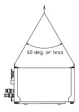
Fig.4.2 How to Lift the Pump
