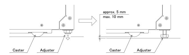
Fig.4.3 Procedure for Adjusting Adjuster
