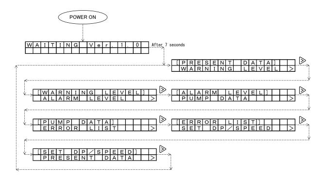
Fig.5.3 The Indication of the handheld Controller
