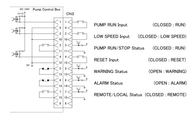
Fig.4.8 CN2 D-sub Connector Pin connections
