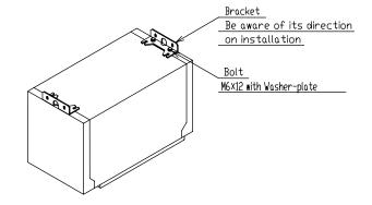
Fig. 4.1 How to install the lifting bracket
