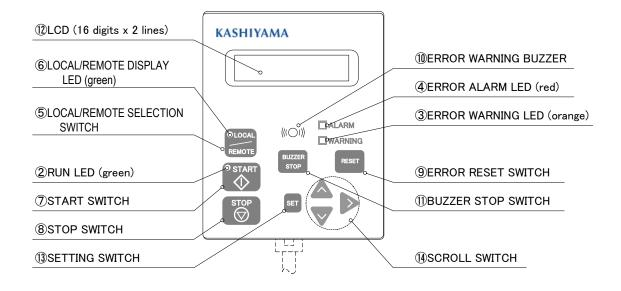
Fig. 5.2 Appearance of the handheld controller
