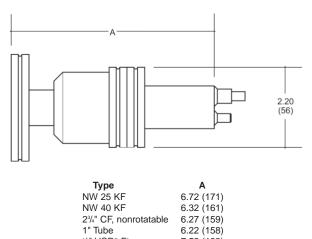
2<sup>3</sup>/<sub>4</sub>" CF, nonrotatable 1" Tube <sup>1</sup>/<sub>2</sub>" VCR<sup>®</sup>-F<sup>1</sup> 7.59 (193) Dimensions: inches (mm)
