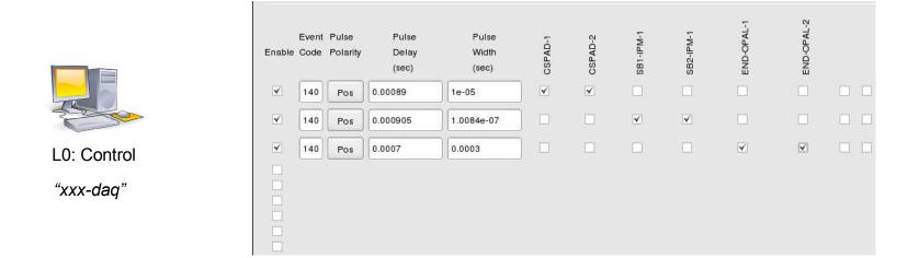
Detector readout is triggered by arrival of an event code (140 = beam on this fiducial) to gate the sampling/digitization with a TTL signal
