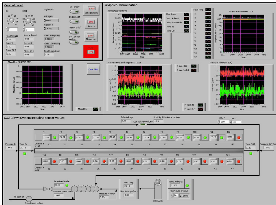
Figure 3.12: Labview front panel interface with on the upper right the power supply controls, adjacently graphs are placed. At the bottom a schematic view of the blown system including sensors values is visible.
