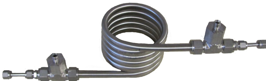
Figure 3.4: Second heat exchanger that is placed after the mass flow meter but before the original heat exchanger.
