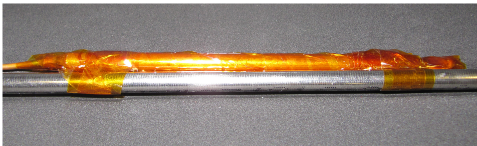
Figure 3.7: Temperature sensor from the power safety box attached to the tube, an electrical isolation layer, is placed in between to prevent a short circuit.
