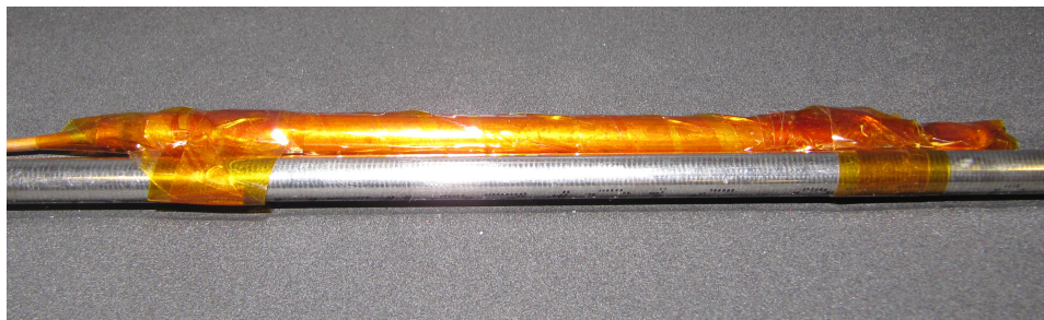
Figure 3.8: Temperature sensor from the power safety box attached to the tube, an electrical isolation layer is placed in between to prevent a short circuit.
