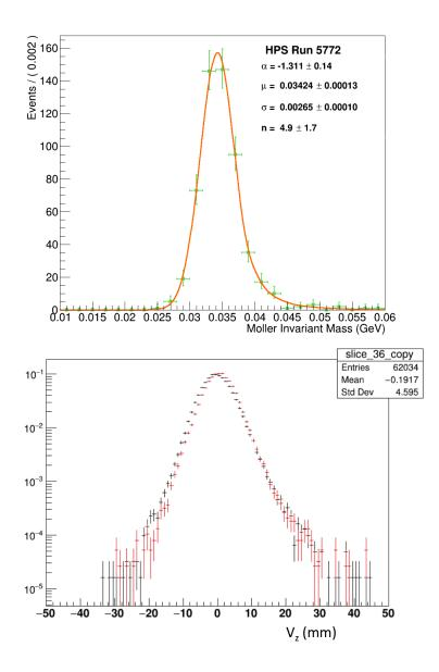
FIG. 5: The invariant mass peak from Moller electrons (top). The distribution of the vertex positions from  $e^+e^-$  pairs along the beam direction for the mass range 38.5 MEV to 42.9 MEV (bottom). Vertex Z = 0 corresponds to the target location; black points are from data and red points are from Monte Carlo..
