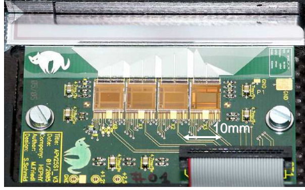
Figure 4.5: A picture of the striplet detector equipped with four APVs.
