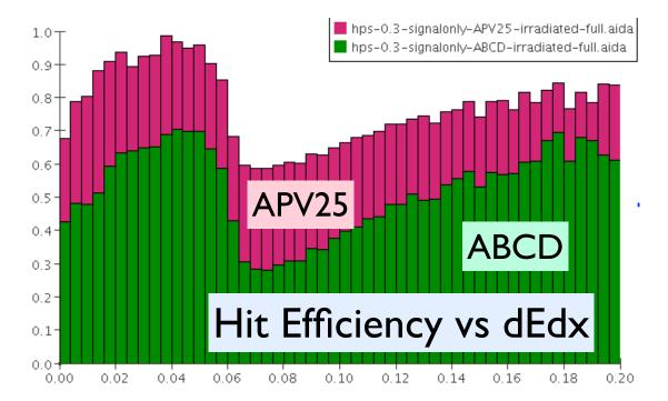
•w/o radiation damage, hit efficiency is >>99%...including it (but not adjusting thresholds) efficiency drops significantly
