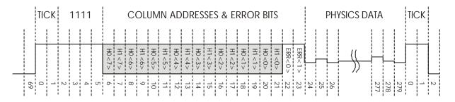
Figure 2-7 APV Frame (40MHz interleaved)
