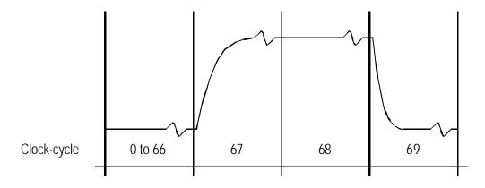
Figure 2-3 Non-ideal waveform of the tick-mark
