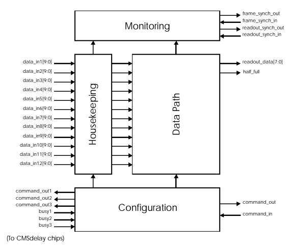
A Block Diagram showing roughly how the Front-End FPGA is laid out is shown below.
