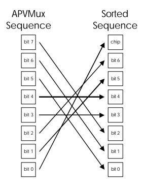
Figure 3-3 APV output bit-swapping sequence
