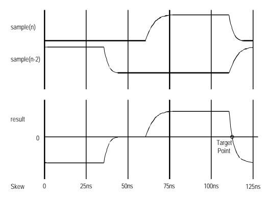
Figure 2-4 Result of averaging the difference between alternate ADC samples
