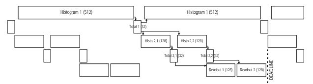
**Figure 3-2 Timing Diagram for Median Calculation**
