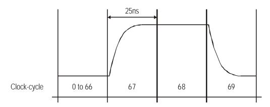
Figure 2-2 Ideal waveform of the Tick-Mark
