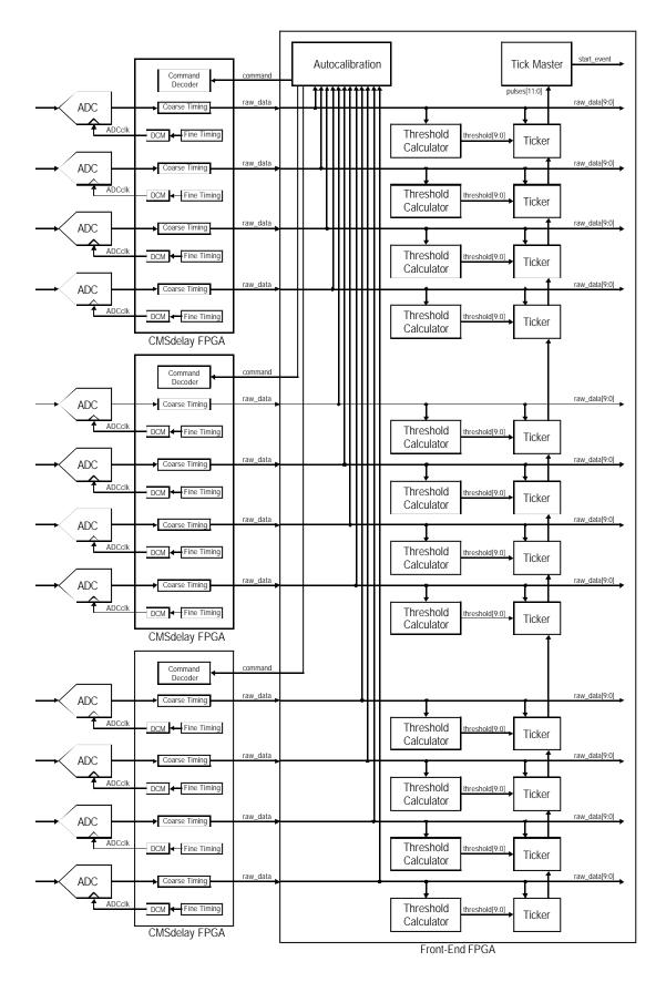
Figure 2-1 Block Diagram of the Housekeeping Components
