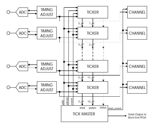
Figure 2-8 Block Diagram showing Tickers and Tick Master
