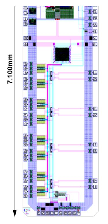
The dimensions of the chip are 2000x7100 microns.
