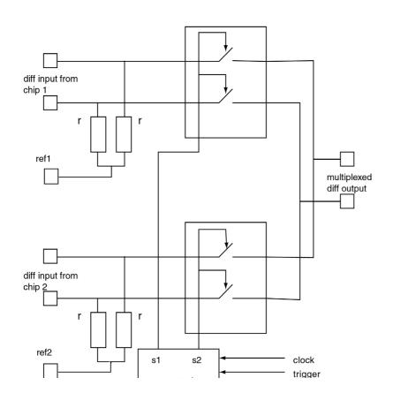
Fig1 schematic of one channel
