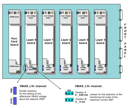
Fig. 3.2 – Divider resistors and jumper settings for the VBIAS\_LY0...4 channels
