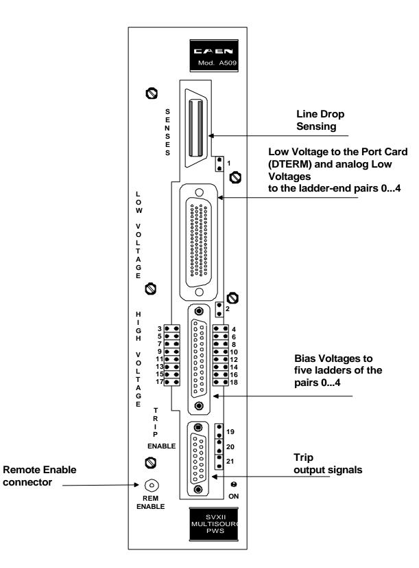
Fig. 2.1 – Front panel of the Mod. A509 Power Supply Board
