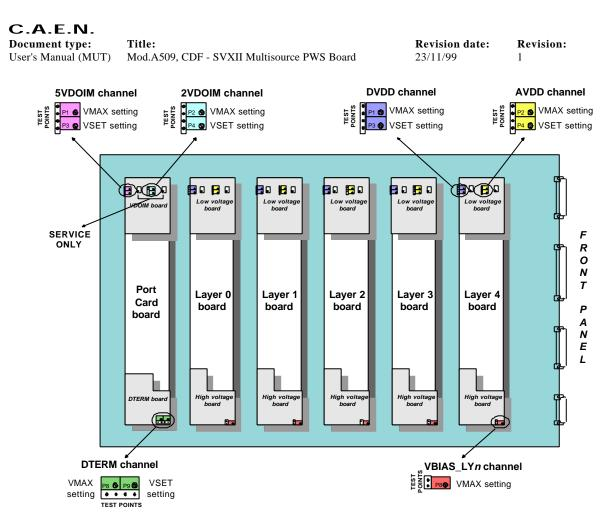
Fig. 3.1 –Trimmer settings for the low voltage channels and the VBIAS\_LY channels
