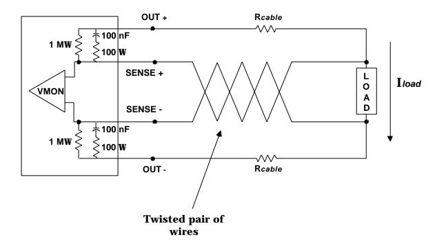
Fig. 4.2 – Voltage Sensing lines
