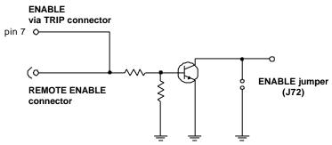
Fig. 4.1 – Electrical diagram of the ENABLE circuitry
