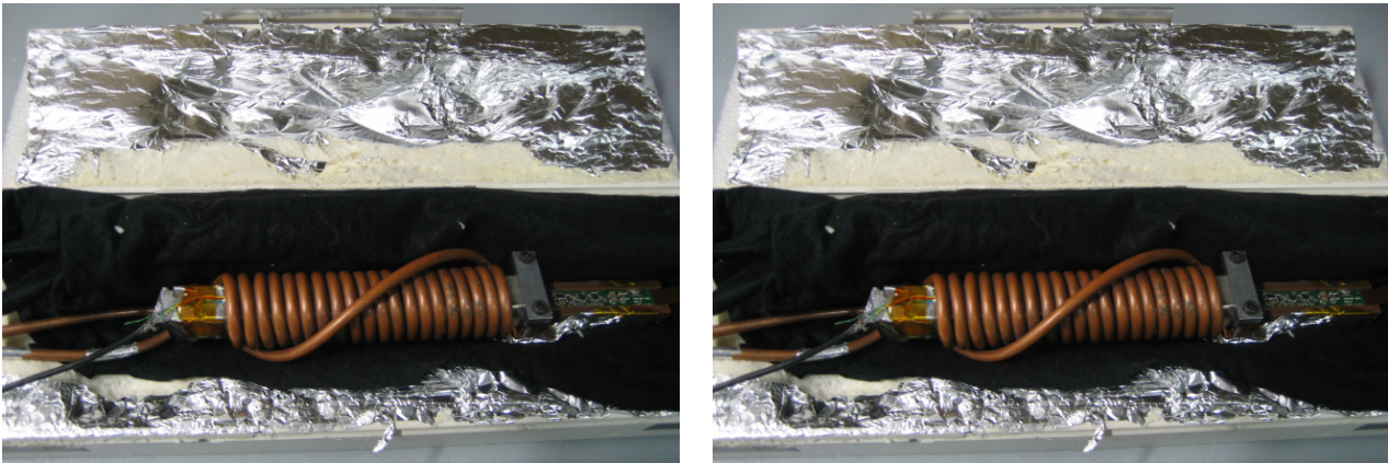
Figure 6: Left: the copper enclosure for light yield measurements. The \text{PbWO}_4 crystal is inserted in the holder between the pipes, and the APD coupled to the amplifier (visible on the right). The external box provides thermal insulation and light tightness. Right: the cosmic ray telescope. The crystal is inserted in between the three counters, horizontally aligned.
