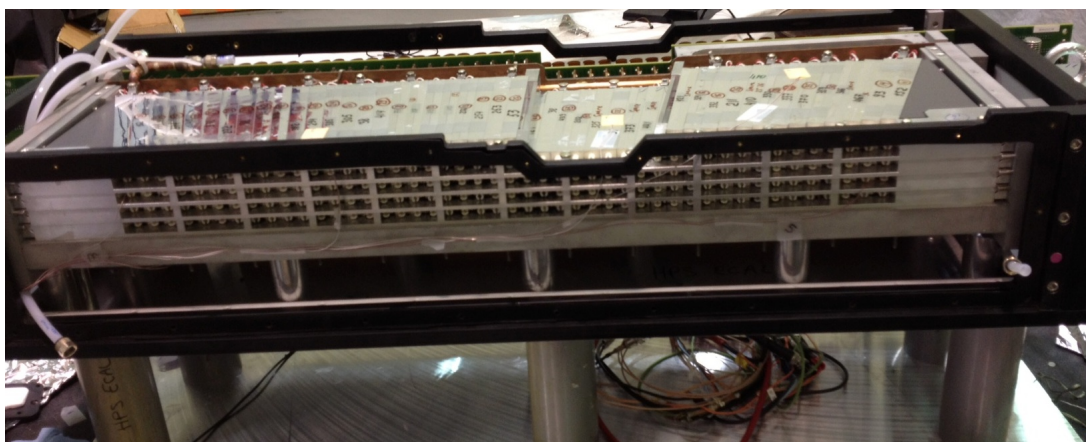
FIG. 34: Assembly of the ECal bottom module.
