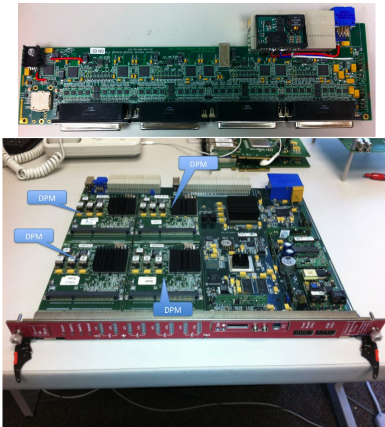
FIG. 38: Picture of a RTM (top) and COB board (bottom) used in the HPS test run 2012.
