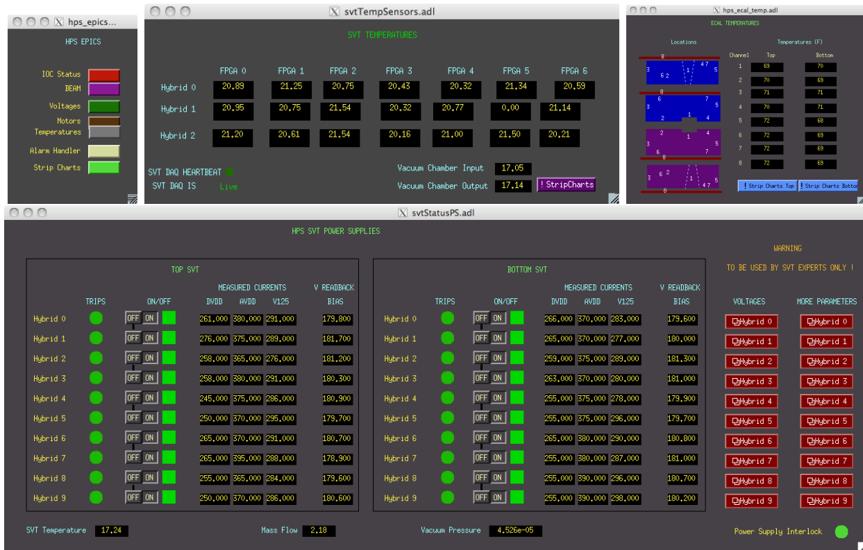
FIG. 14: Voltage and temperature control screens during 2012 test run in Hall B. Similar control screens will be developed for 2014 run using CSS BOY display management framework.
