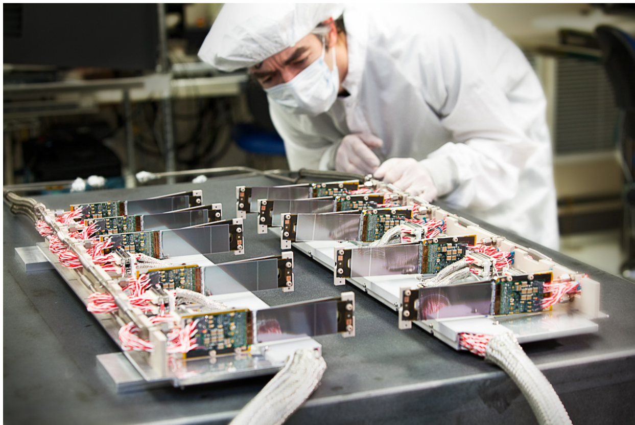
FIG. 33: Both halves of the HPS Test SVT fully assembled at SLAC.
