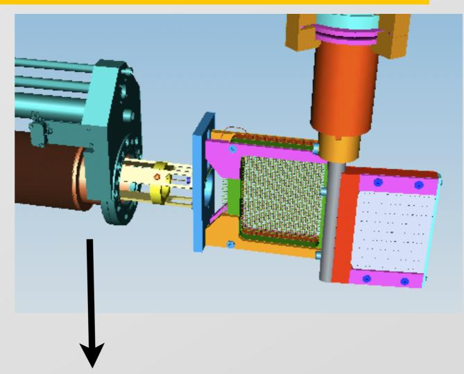
(JLAB designed) active sieve slit for optics calibration: 2-layer (xy) scintillating fiber detector. Improve the efficiency & reliability of optics calibration.
