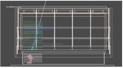
The green crosses show the detected positions of the charged particles, the blue lines show the reconstructed track trajectories, and the yellow line shows the candidate gamma-ray estimated direction. The red crosses show the detected energy depositions in the calorimeter.
